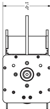
End plate bolts to industry standard 12"x12" truss.
